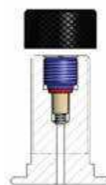
Model of valve stem integrated 5/8" 18 UNF (D)
