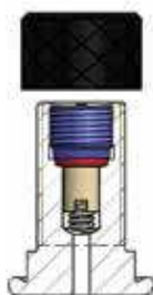
Model of valve stem integrated 7/8"14 UNF (C)
