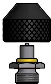
Model of valve stem 7/8" 14 UNF (B)
