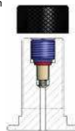
Model of valve stem integrated 5/8" 18 UNF (D)
