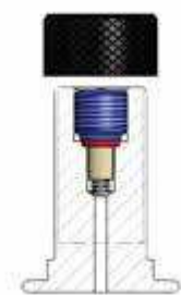
Model of valve stem integrated 5/8" 18 UNF (D)
